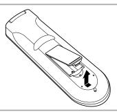
2 Install 2 batteries ("AAA" size) following the polarity diagrams.
